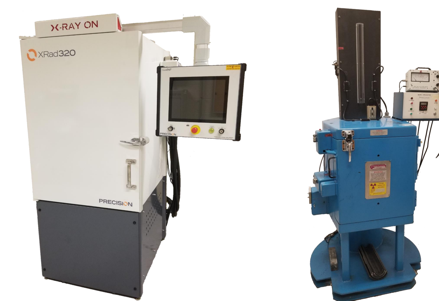
The x-ray irradiator (left) and the \gamma -ray irradiator (right) used
